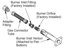
Figure 6 - Connecting Gas to Appliance
